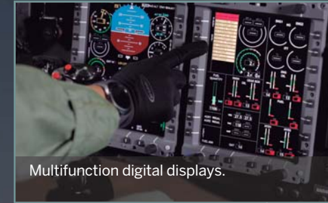
GTN 750 navigation system. High Terrain Approach Warning System (HTAWS).
