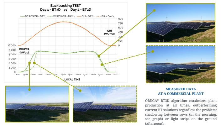
Outperforming all competitors so far, ORUGA® 3D Backtracking increases plant production when electricity price is at its highest: in the morning and in the afternoon.
